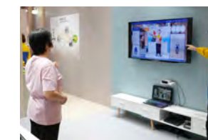
擴增實境復康訓練系統，實時監控患者在治療運動時的肢體動作，協調訓練及表現。 The augmented reality rehabilitation training system can monitor a patient's body movement, coordination and performance in real time.
