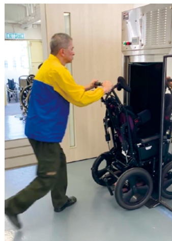
專業人員將使用後的輪椅放入消毒乾燥機進行全面消毒。 Used equipment is thoroughly sterilised in a disinfection and drying machine.
