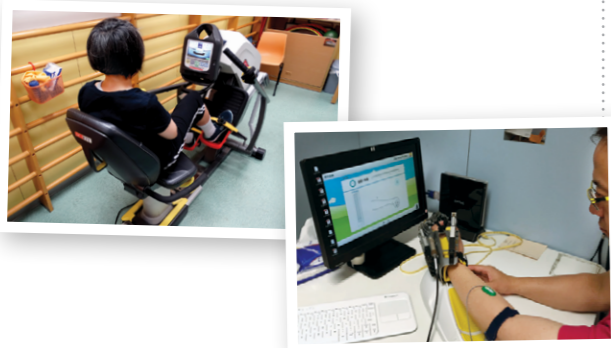
中心去年度添置了不同復康器材，如肌電驅動穿戴式機械手「希望之手」(右)及下肢肌力訓練儀(左)。 The Centres last year procured various rehabilitation equipment such as "Hands of Hope", an EMG-driven exoskeleton hand robotic training device (right) and the Recumbent Stepper for training lower body muscles (left).
