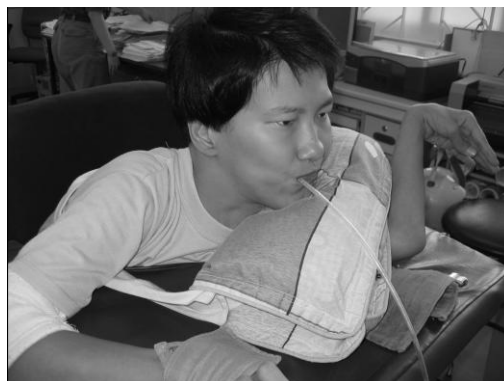
Figure 4: Pui Ling using a suck-and-blow input device for controlling her computer.
