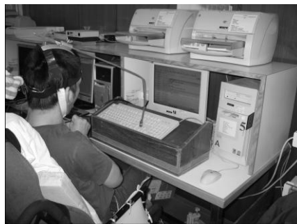
Figure 5: “Sky” using a head point as input device for controlling his computer.
