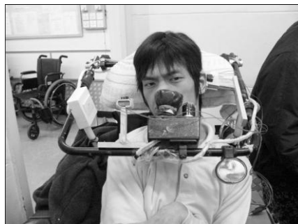
Figure 6: “Sky” controls his power wheelchair with a chin control device.
